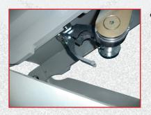
"Crocodile" device added to stop lift in case of misalignment
